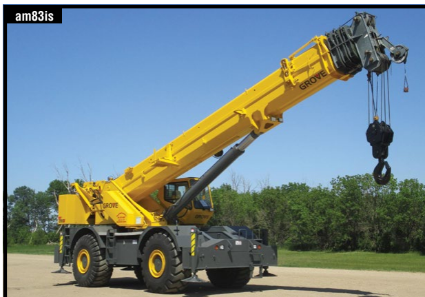
am83is 2006 GROVE RT890E S/N: 225533, 6994 Hrs, 90 Ton Rough Terrain Crane, 38' - 142' Five -section full power boom, 33' - 56' bi-fold lattice ..... CALL FOR PRICE
