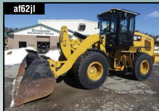
af62jl 2012 CAT 930K Stk # LO556, 2247 hrs, 3.5 yard, cab w/ a/c, hyd coupler w/ 3rd valve, 6 cyl cat turbo, good rubber, 31k lb size class . . . . . $133,950
