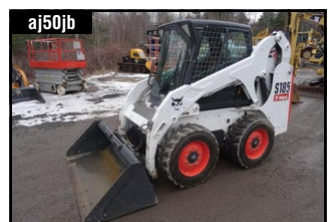
aj50jb 2012 BOBCAT S185 Stk # SK657, 549 hrs, 1850 lb lift, cab w/ a/c, aux hyd, mech cplr, 4 cyl kubota turbo, 66" bucket, 6.5k lb lbs . . . . . $29,900
