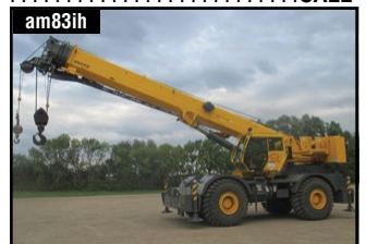
am83ih GROVE RT765E-2 S/N: 232390, 65 Ton Rough Terrain Crane, 36' x 110' four-section full power boom ... CALL
